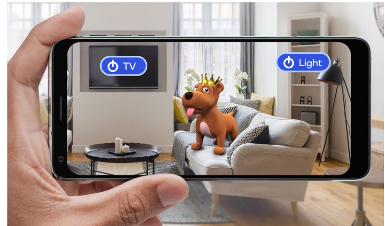
Figure 2: Advanced AR showing digital content (dog character) anchored to a physical object (couch).
